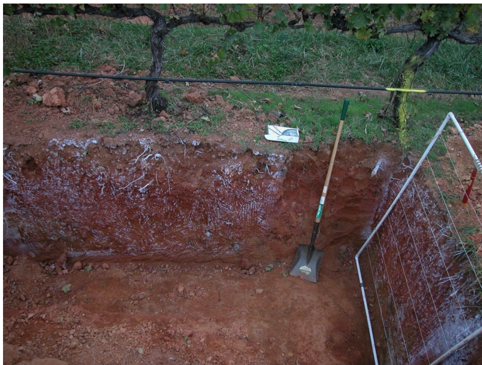
Figure 5.2 Perpendicular and parallel soil pit faces, painted with roots exposed and subquadrat grid in place on perpendicular face prior to counting root intercepts within each subquadrat.
