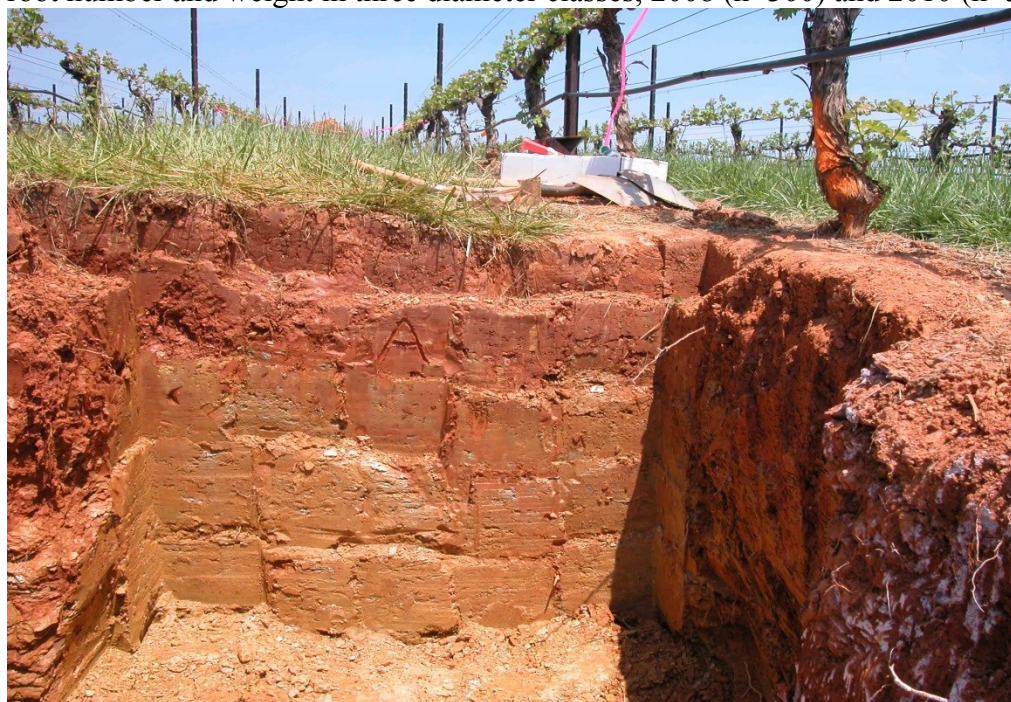
Figure 5.4 Perpendicular soil pit face after sequential removal of twenty-five soil block samples for root count and biomass determination.
