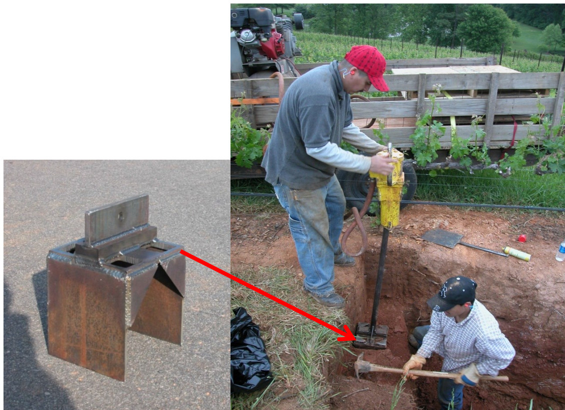
Figure 5.3 Soil probe (8000 cm 3 ) used for extraction of soil sample blocks and determination of root number and weight in three diameter classes, 2008 (n=300) and 2010 (n=300).
