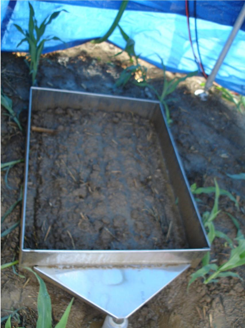
*Figure 1 Steel weir frame used to isolate runoff for delivery to covered flume for collection.*
