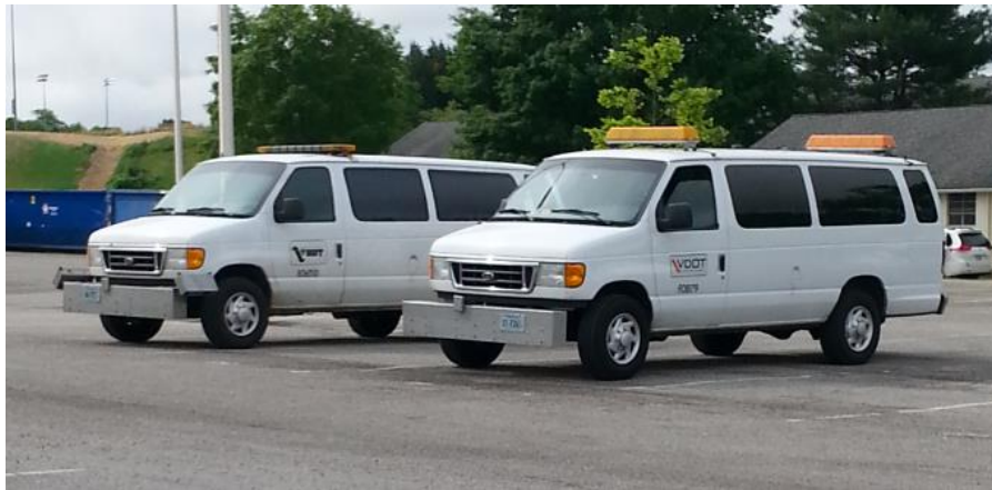
Figure 1. Illustration of current inertial road profilers
