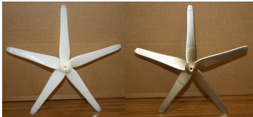
Figure 6.6 Prototype ingress vehicle propeller. ABS (left) Nickel and Copper plated ABS (right)
