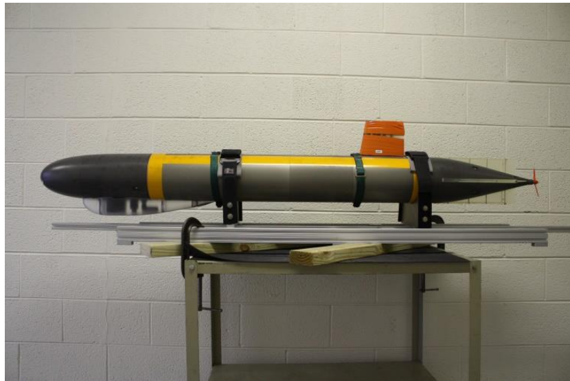
Figure 2.2 Virginia Tech Self-Mooring AUV shown without the false nose, which functions as a mooring anchor
