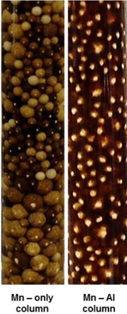
Figure 2.12. Appearance of two columns with alumina spheres used as media at the end of experiments (sixth day). Media was exposed to Mn^{2+} in the absence and presence of Al with free chlorine as oxidant across the filter.
