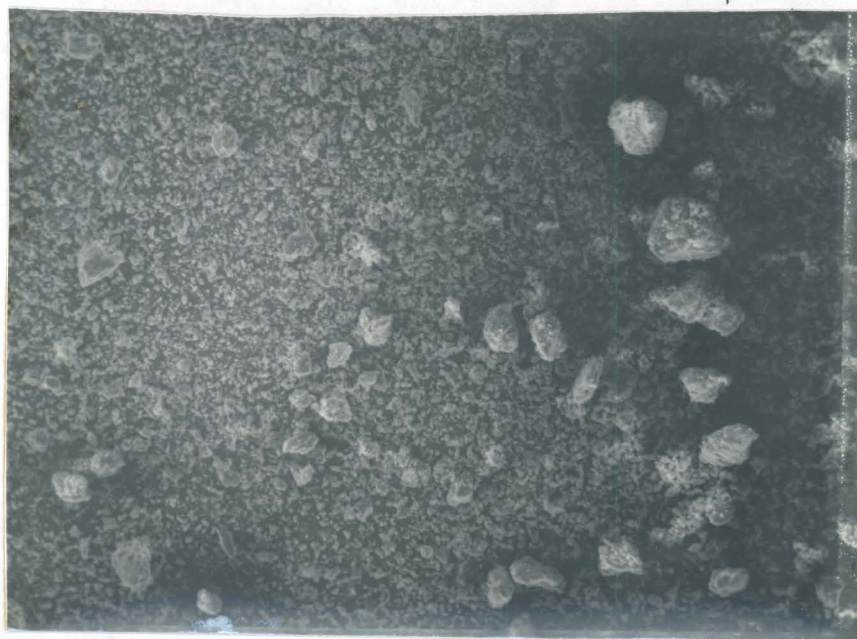
Figure A-2. Size Comparison of Photomicrographs of Illinois No. 6 Coal Samples Ground for (a) 15 Minutes and (b) 20 Minutes, Magnified 100 Times. Note: AMR Model 900 Scanning Electron Microscope was Used.
