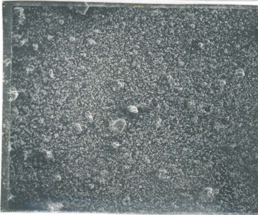
Figure A-4. Size Comparison of Photomicrographs of Illinois No. 6 Coal Samples Ground for (a) 50 Minutes and (b) 60 Minutes Magnified 100 Times. Note: AMR Model 900 Scanning Electron Microscope was Used.
