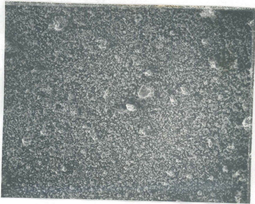
Figure 5.2. Size Comparison of Photomicrographs of Illinois No. 6 Coal Samples Ground for (a) 5 Minutes and (b) 60 Minutes, Magnified 100 Times. Note: AMR Model 900 Scanning Electron Microscope Was Used.
