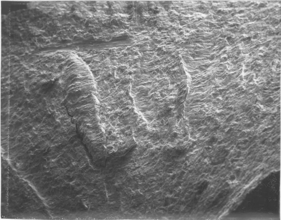
FIGURE 16. FRACTURE SURFACE OF A HYDROGEN-CHARGED SPECIMEN SHOWING NO STRIATIONS. 180X (High humidity 16,800 psi 117 MPa stress)
