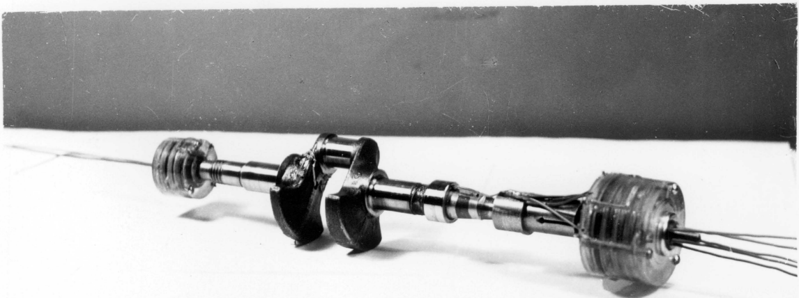
FIG. 16 The construction of the liquid-to-solid slip-ring units
