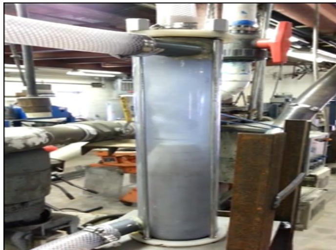
Figure 4.1. Development of Air Core in Initial Flotation Cyclone.
