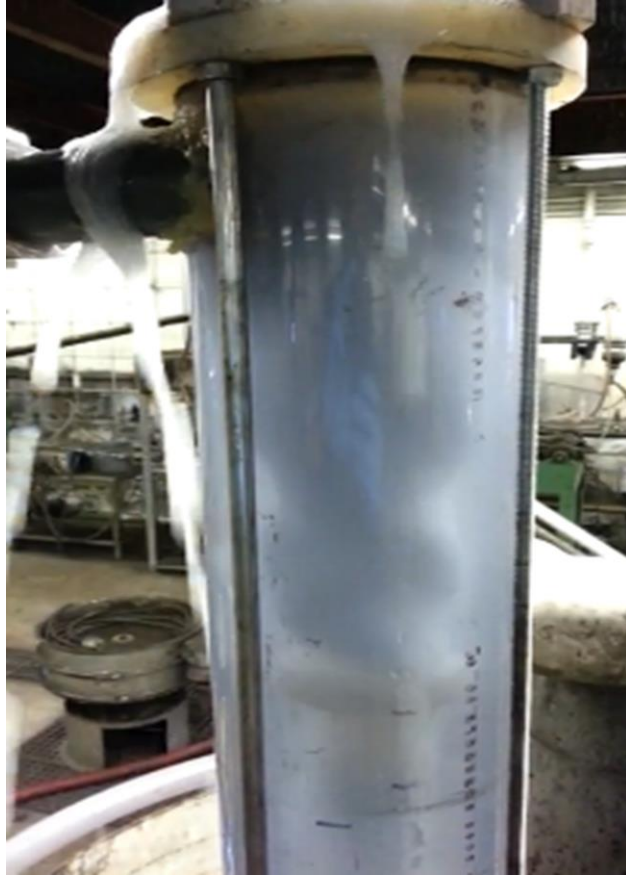
Figure 3.3. Flotation Cyclone with Adjustable Pedestal and Two U/F Streams.
