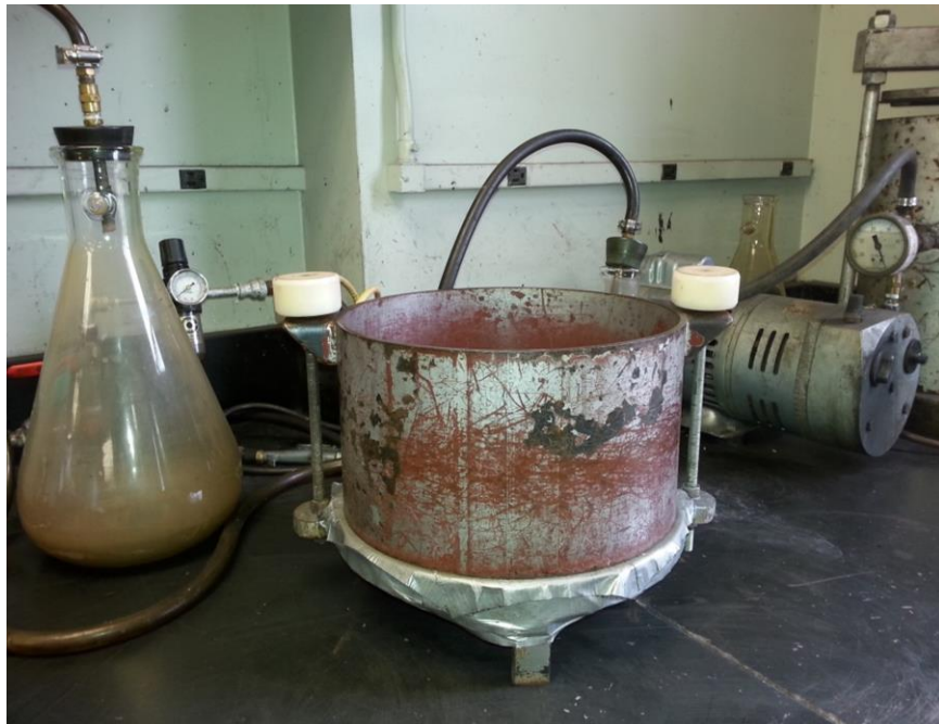
Figure 3.8. Vacuum Pump Dewatering Configuration
