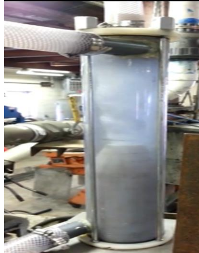
Figure 3.2. Initial Flotation Cyclone Design in Operation.
