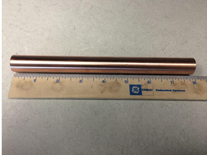
Figure 3-9 Final selection of heat pipe
