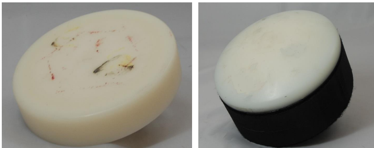
Figure 10. Polymer caps for linear impactor. Left: Flat impactor, Right: Curved padded impactor.
