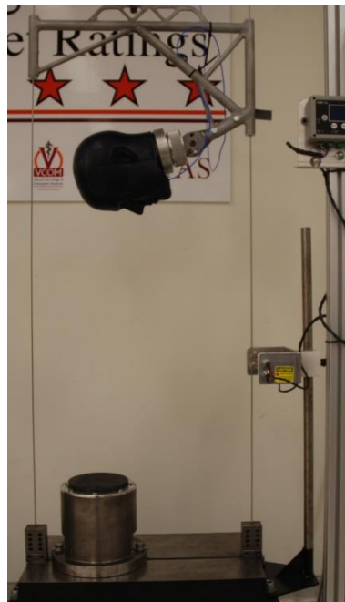
Figure 8. NOCSAE twin-wire guided drop tower with MEP pad, carriage assembly, and NOCSAE headform.
