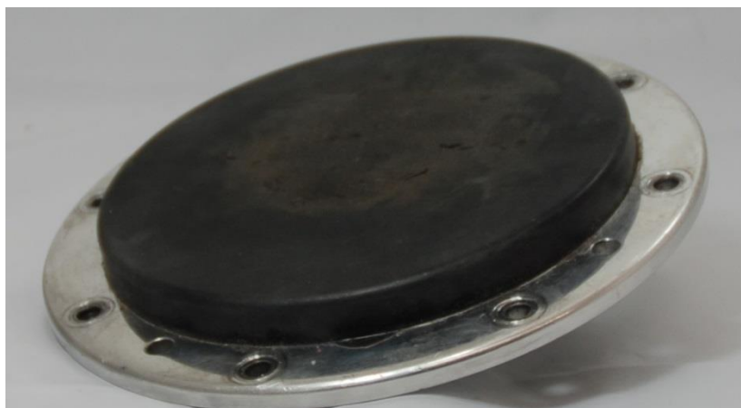
Figure 7. NOCSAE thermoplastic polyurethane MEP pad.
