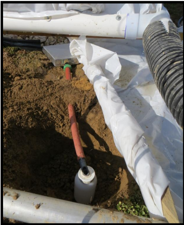
Figure 3.5. Runoff collection pan and bottle.
