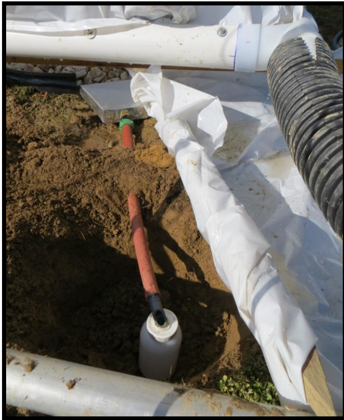
Figure 3.2. Runoff collection pan and bottle.
