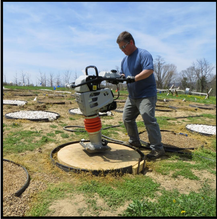
Figure 3.3. The compaction treatment was performed by running a jumping-jack style compactor over a 38 mm thick plywood disk on each plot. The disk was slightly smaller than the plot to avoid disturbing plot borders.
