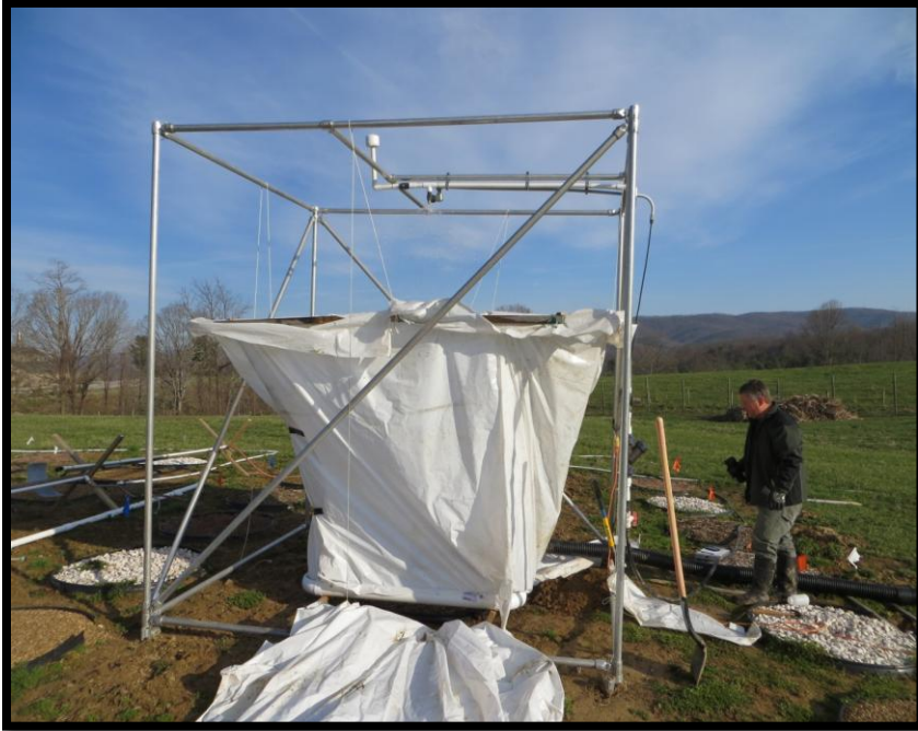
Figure 3.4. Plastic sheeting was used to isolate experimental units during rainfall simulation and shield adjacent plots from overspray. The sheeting also piped excess water out of the work area.
