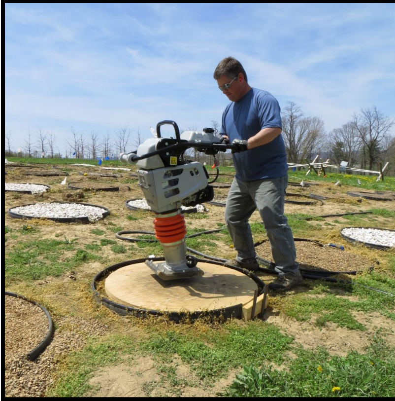
Figure 6.3. The compaction treatment was performed by running a jumping-jack style compactor over a 38 mm thick plywood disk on each plot. The disk was slightly smaller than the plot to avoid disturbing plot borders.
