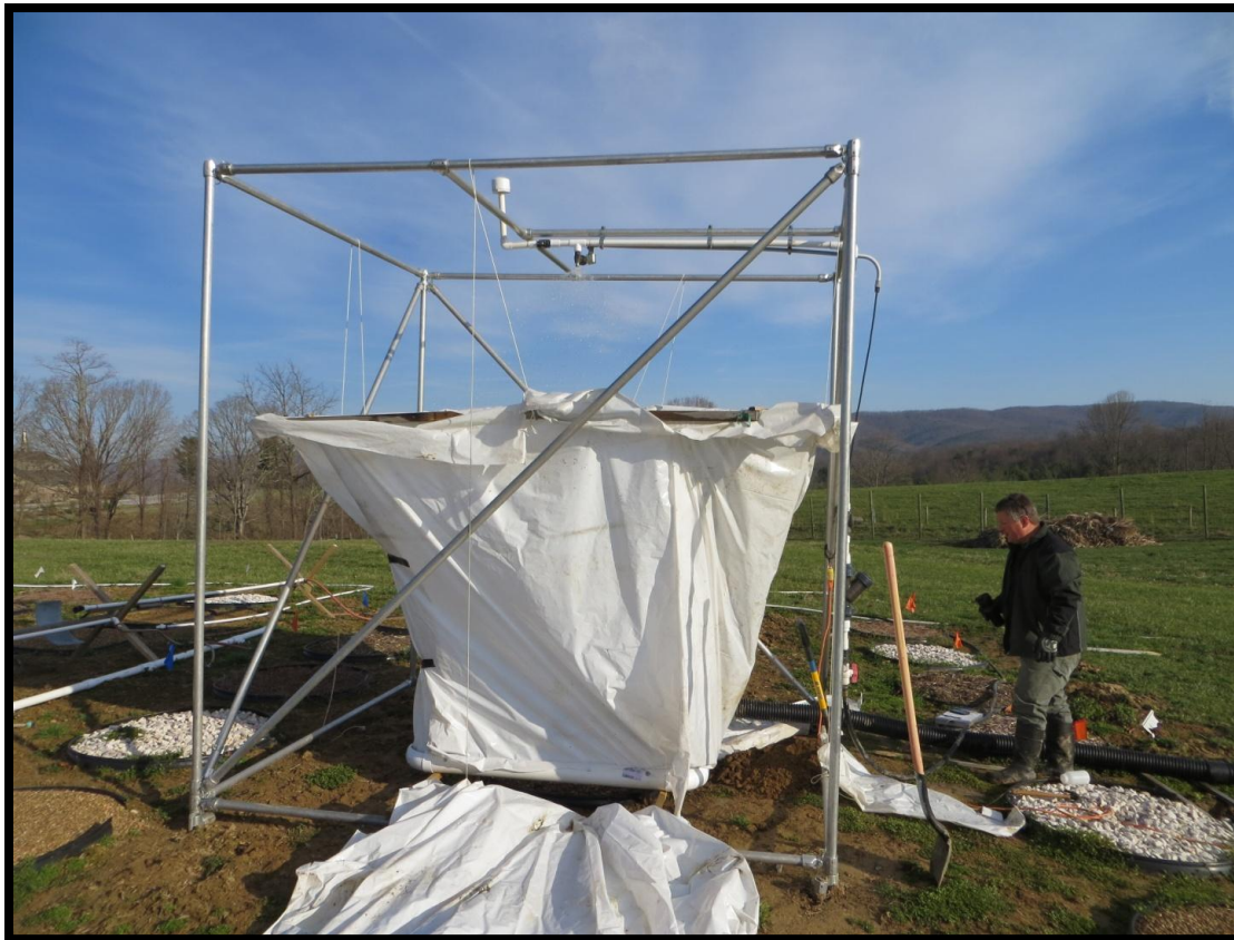
Figure 3.1. Plastic sheeting was used to isolate experimental units during rainfall simulation and shield adjacent plots from overspray. The sheeting also piped excess water out of the work area.
