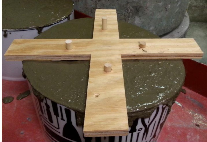
Figure 3-1: Placement of tubes in wet concrete
