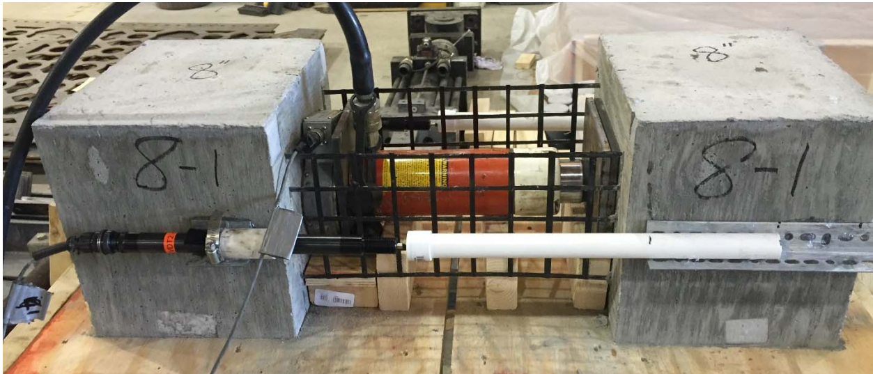
Figure 14: Development Length Instrumentation
