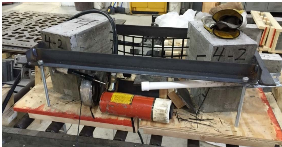
Figure 13: Typical Development Length Failure
