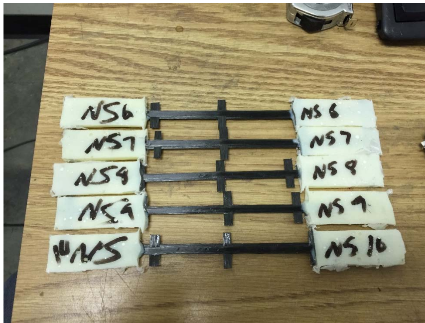
Figure 8: Tensile Strength Specimens
