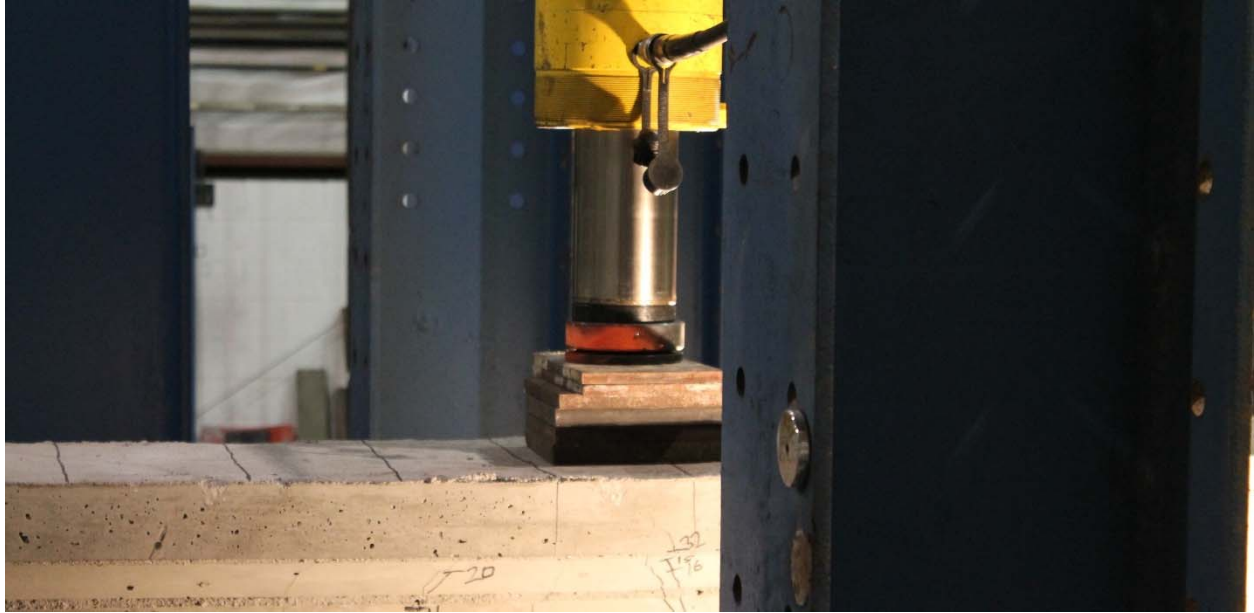
Figure 23: Loading Plates under Hydraulic Ram
