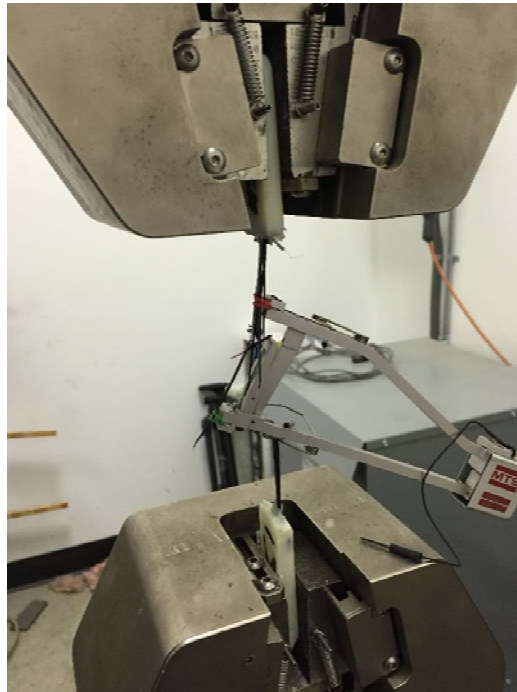
Figure 10: Typical Failure of Tensile Specimen
