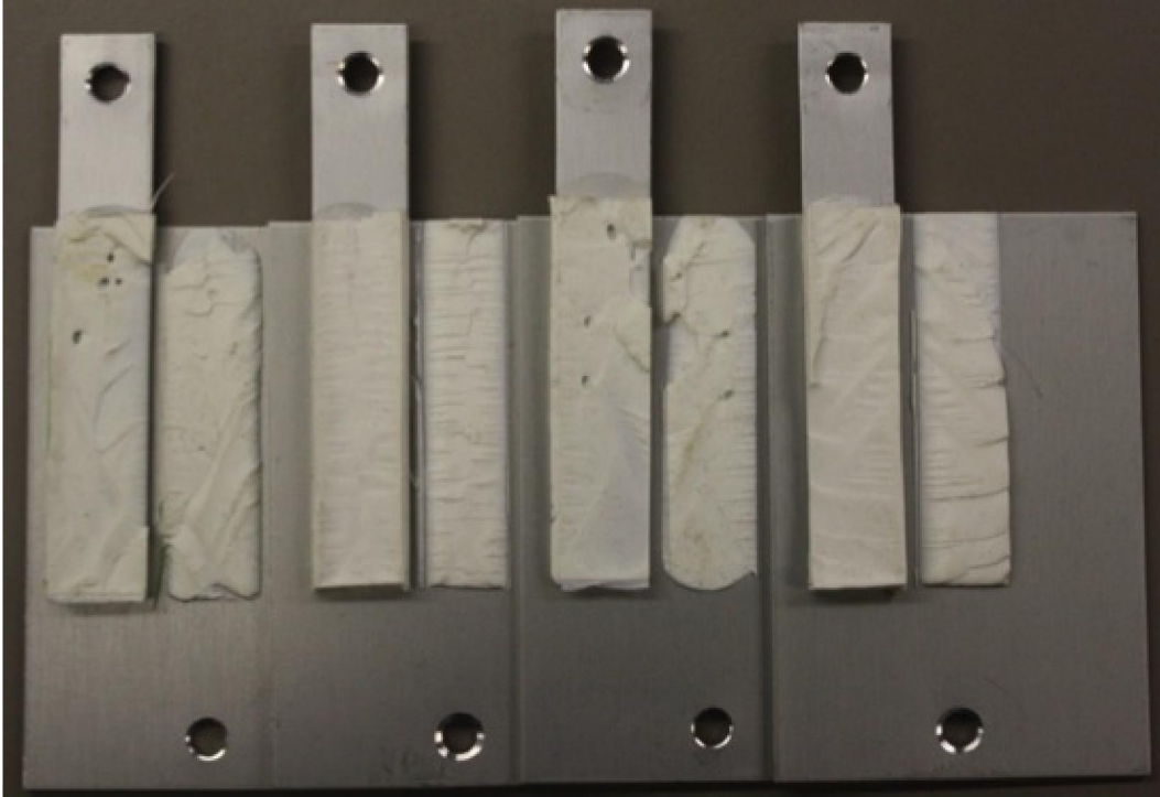
Figure 5-25: Representative failure surfaces of Al-Al specimens from creep rupture tests at 30°C and middle stress level (0.61 MPa)
