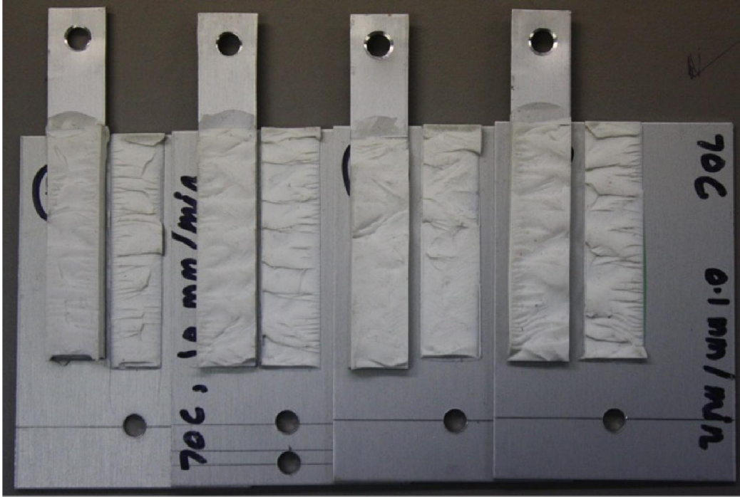
Figure 5-12: Representative failure surfaces of specimens from ramp to fail tests at 70°C and 3.2 s -1 , 0.32 s -1 , 0.032 s -1 , 0.0032 s -1 strain rates (from left to right) on sealant C
