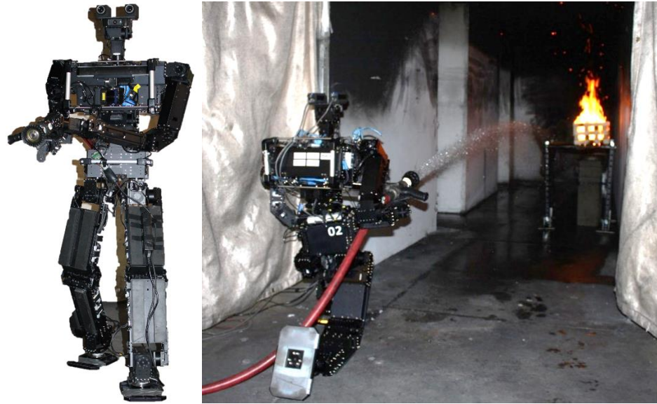
Figure 1. A prototype of Shipboard Autonomous Firefighting Robot (SAFFiR)
