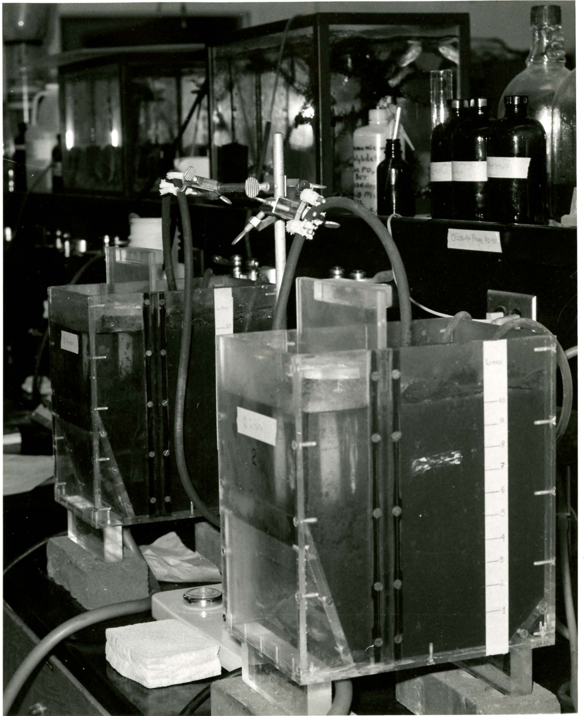
Figure 3. Bench Scale Activated Sludge Plant.
