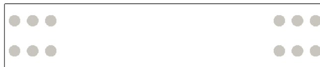
Figure 3.9: Cross-sectional view of shear wall, showing the layout of the 12.5 mm diameter steel reinforcing bars
