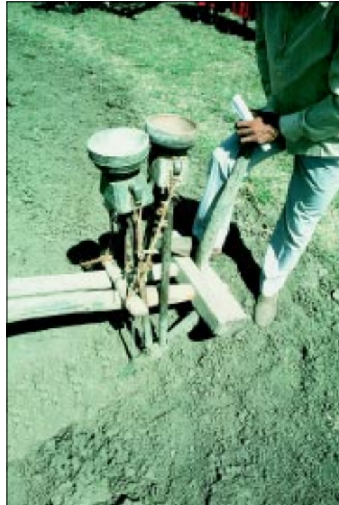
PLATE 70 It was demonstrated to the farmers that better germination occurred when the fertilizer was banded 1 cm or so below the line of seeds, and that this could be done with a commercially-manufactured combine seeder. The village blacksmith, however, said he could modify the existing seeders to do the same job without much cost or difficulty. The fertilizer on its own is placed down the forward spout and falls slightly in front of and below the seed, which falls down the rear spout [T.F. Shaxson]
