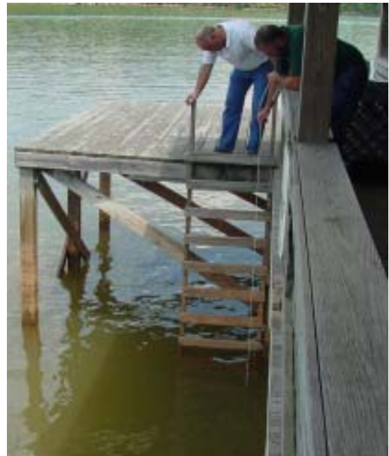
Tom Hoggle and Larry Raughton measure lake water clarity using a Secchi Disk
