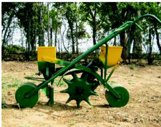
Photo 7. Manual drawn star wheel multi crop no-till planter.
