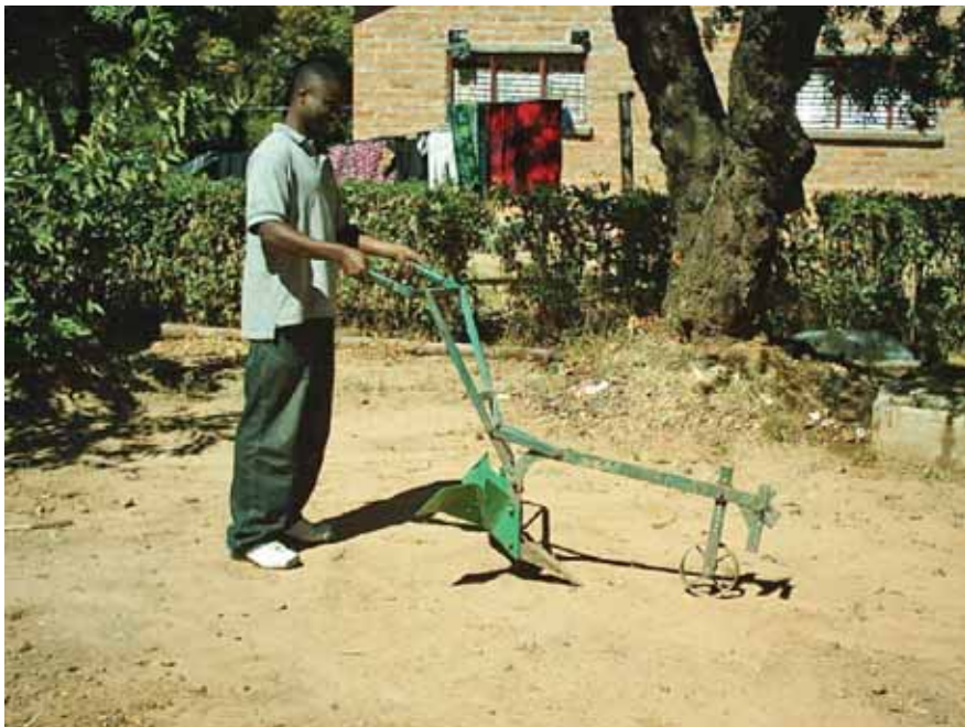
The Magoye ripper with extended wings
