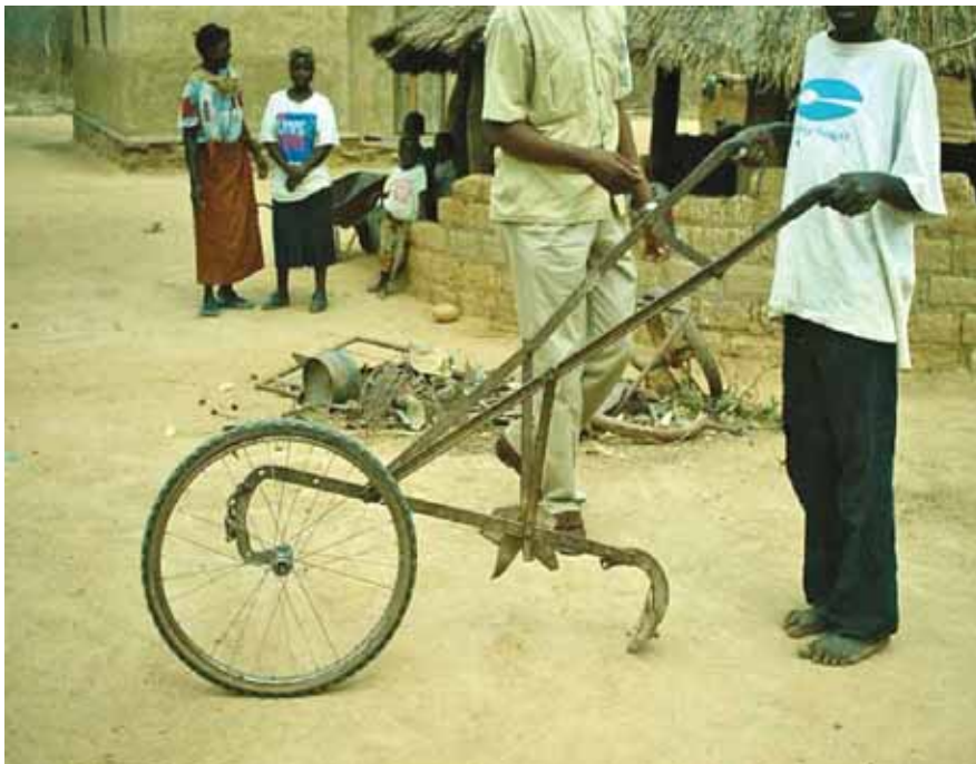
A local man-pulled adaptation of the ripper
