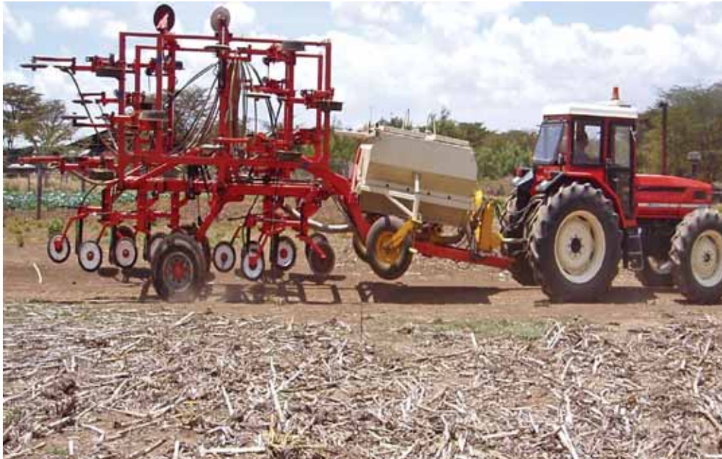
No-till pneumatic direct seeder on display at Lengetia Farm
