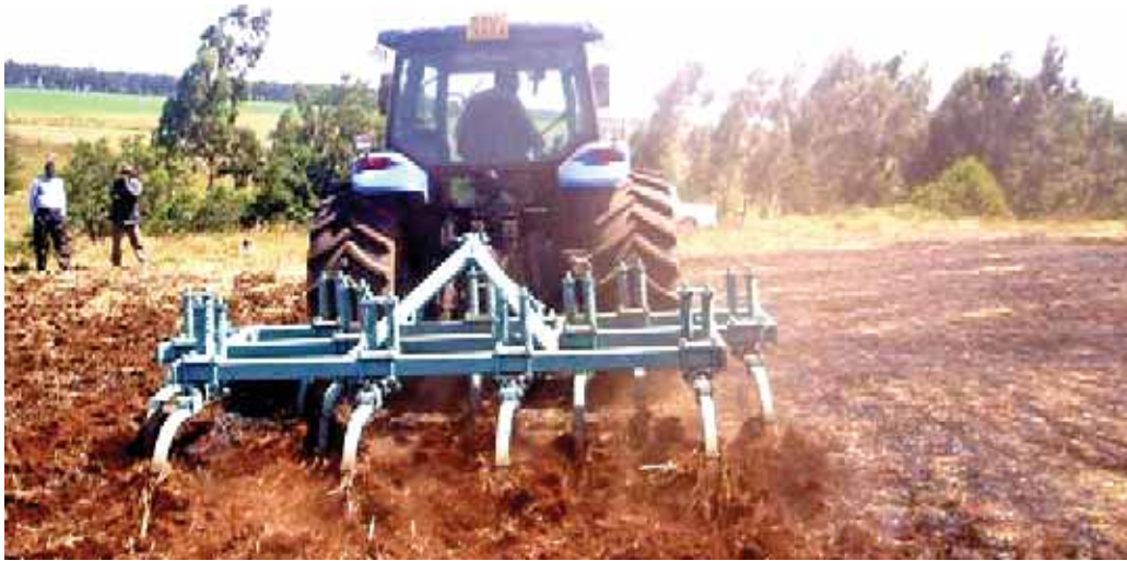
Heavy tine harrow implement operating on Wangu Farm
