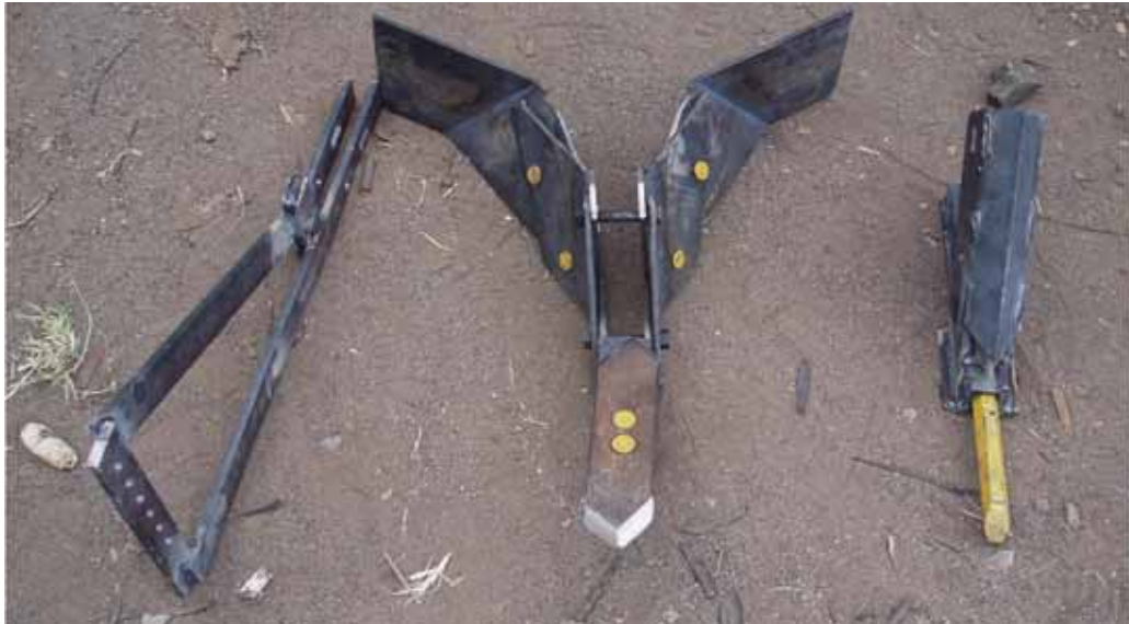
Locally manufactured Magoye ripper and subsoiler, which can fit onto the same frame as the plough
