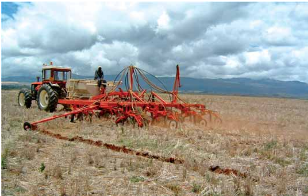
No-till pneumatic direct seeder in action on one of the Lengetia fields
