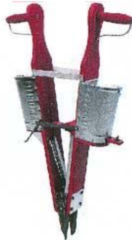
Figure 2.6 Hand-jab Planter (No-tillage drill and planter design - small scale machines) [9]
