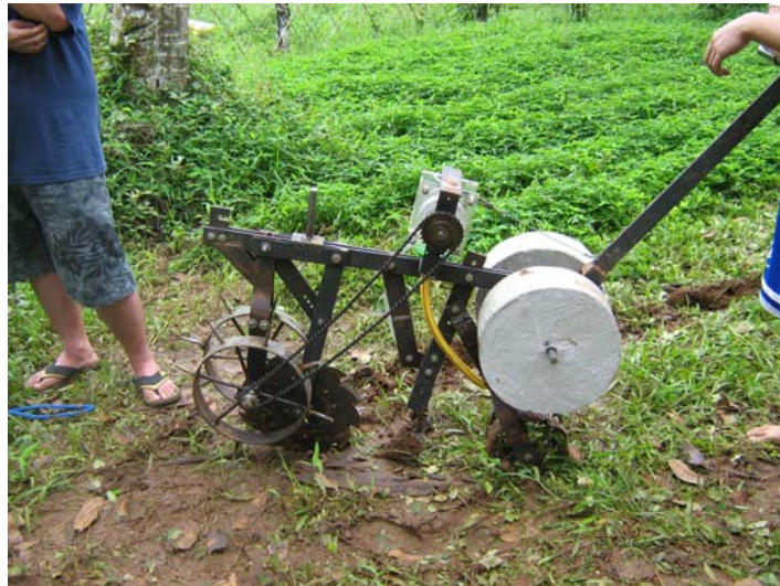
(b) No-Till Equipment with added weights
