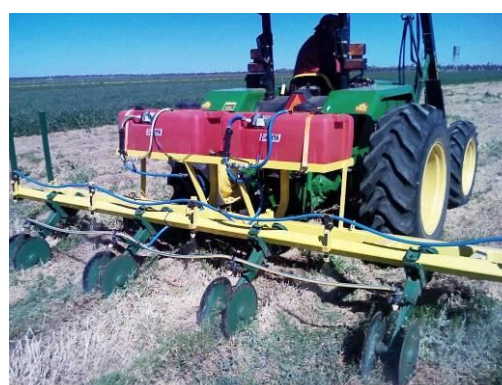
Figure 2. Final design ("Stage 3") of mulching implement
