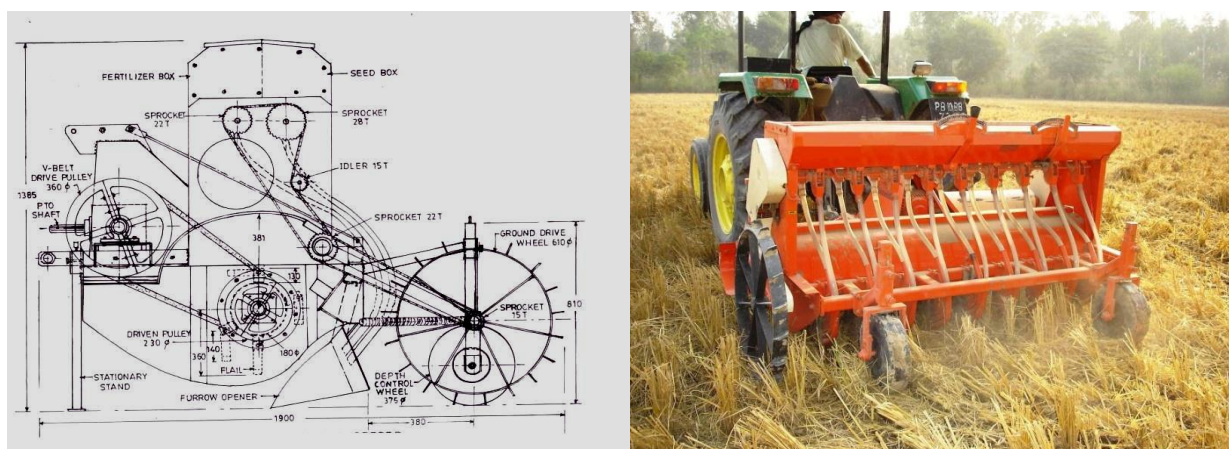
Figure 1. Side View of Turbo Happy Seeder with Technical details and machine in operation
