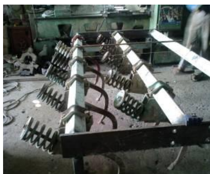
Plate 9: Fabrication of local 2.3 m ZT seeder
