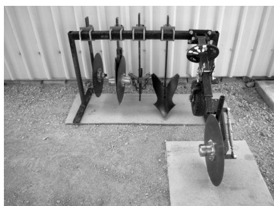
Figure 3. Some optional soil engaging tools to fit the tined seed drill
