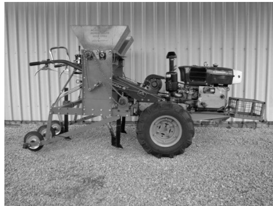
Figure 2. The improved ACIAR-Rogro tined seed drill
