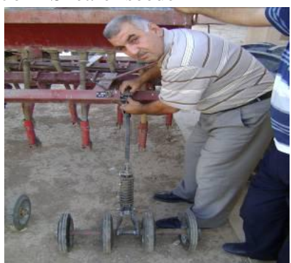
Plate 5: Locally made gang of 4 presswheels
