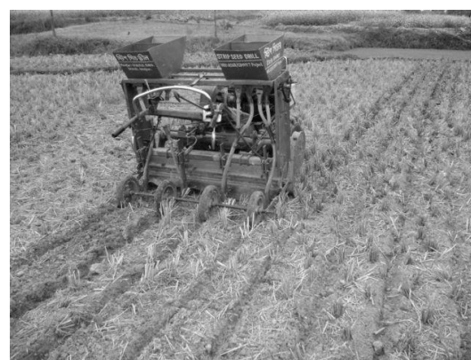
Figure 4. A Bangladeshi made rotary tillage feed drill set up in strip tillage mode.
