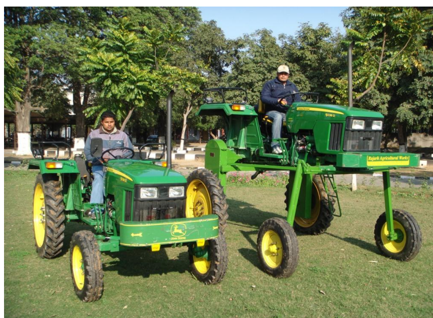
Figure 2. High clearance platform for 4-wheel tractor
