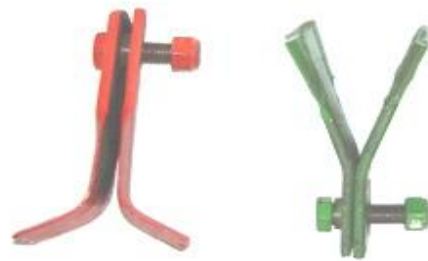
Figure 1. J-type and Gamma-type flail blades used in HS
