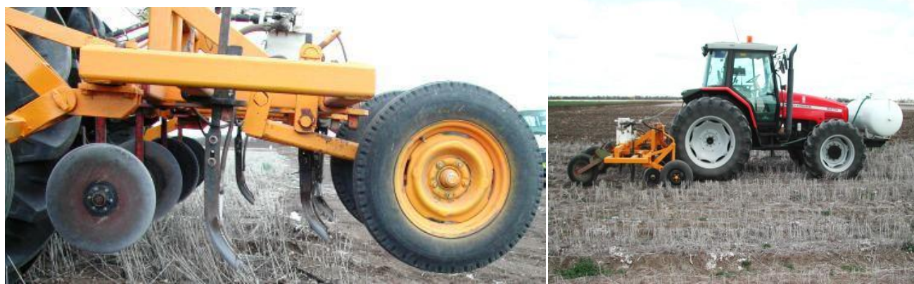
Figure 3. Modified gas (anhydrous ammonia) rig with coulters in front of gas knives
