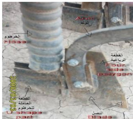
Plate 2: First prototype ZT opener
