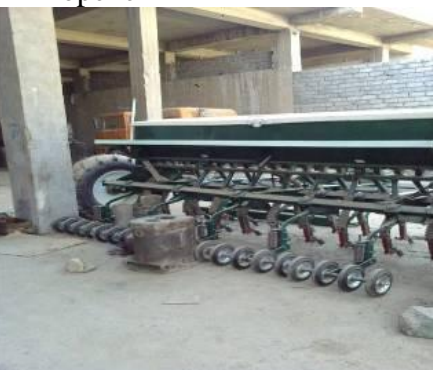
Plate 6: Local 3.6 m seeder converted for ZT with press wheels
