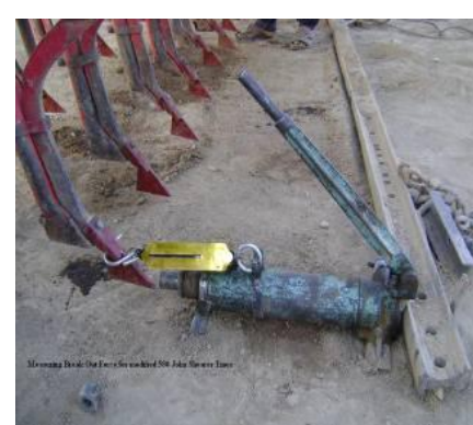
Plate 4: Local testing of tine breakout force
