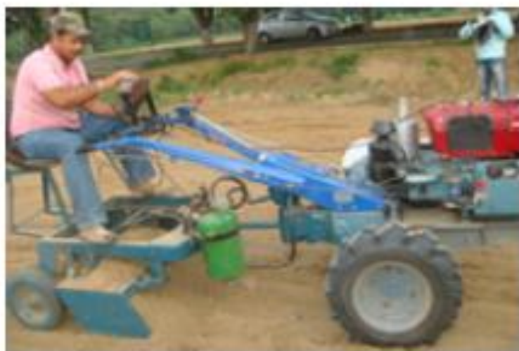
Figure 3. Two Wheel Tractor Based Laser Land Leveler
