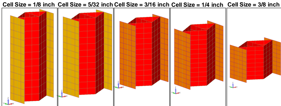
Figure 4-5: Unit cell models for triangular core
