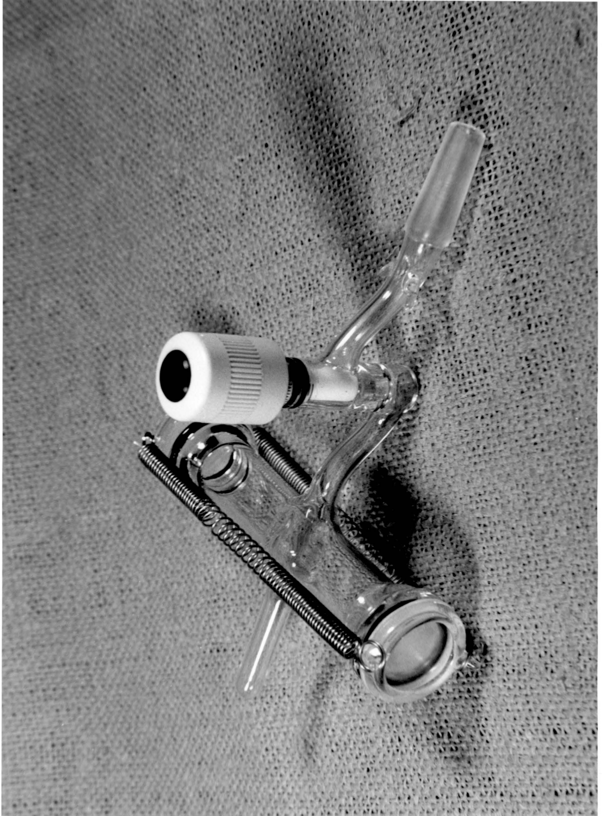
Photograph 1. Infrared Gas Cell
