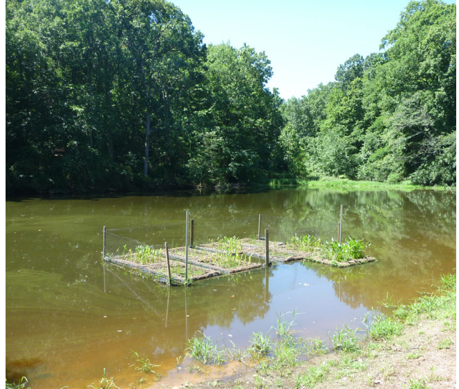
Figure 2. Floating treatment wetland (FTW) rafts in Ashby Pond, Fairfax, Va.
