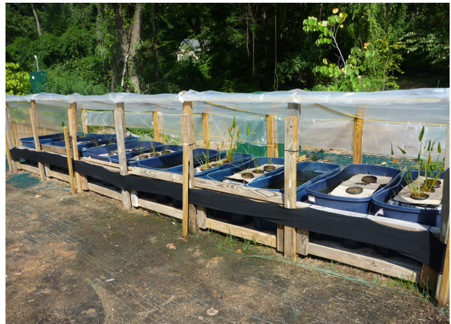
Figure 4. Floating treatment wetland mesocosms, Fairfax, Va.
