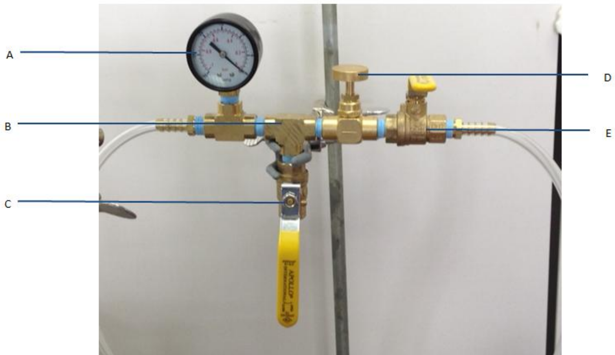
The gas outlet set-up for the Ethanol Vapor Apparatus. A) Vacuum gauge with barb attachment; B) T joint; C) ball valve; D) needle valve; E) ball valve with barb attachment
