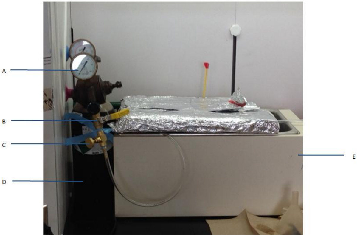
Nitrogen gas input for the Ethanol Vapor Apparatus. A) Nitrogen gas regulator; B) brass ball valve; C) brass needle valve; D) compressed nitrogen gas; E) water bath with thermometer, custom lid and quarter inch diameter copper tubing coiled connected to quarter inch interior diameter surgical tubing.
