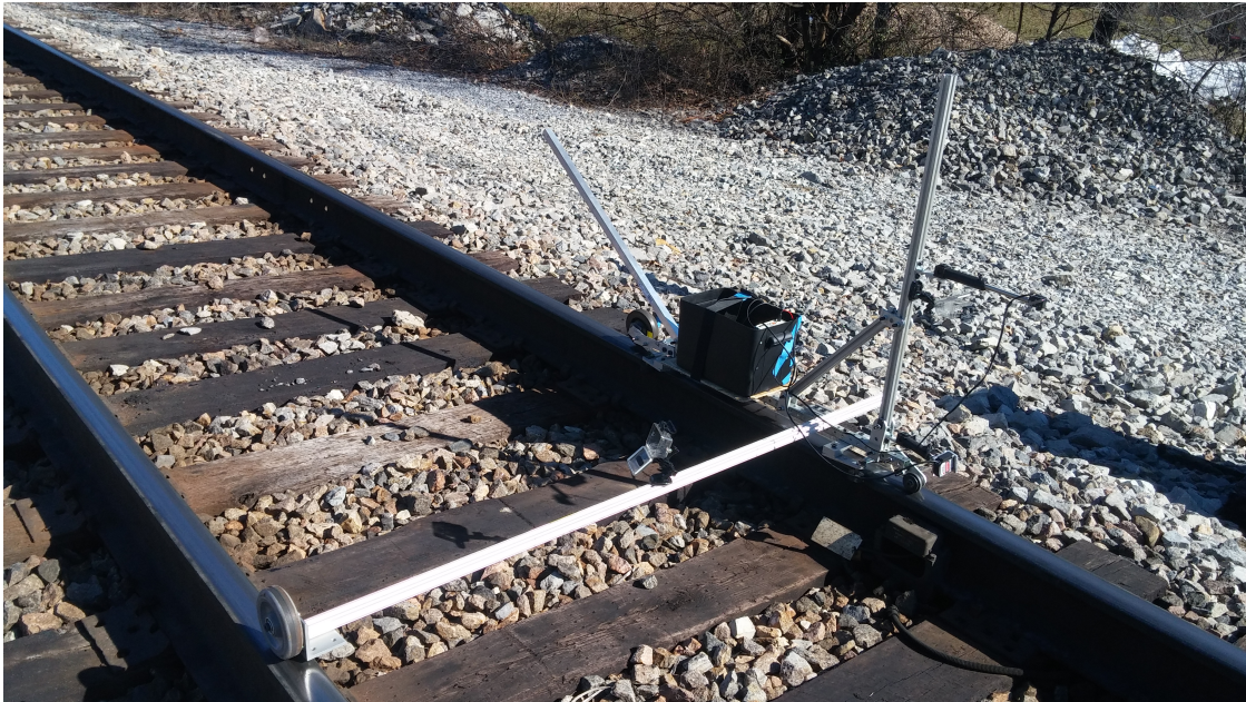
Figure 6-4 Modified cart equipped with laser sensor, encoder, and data acquisition system
