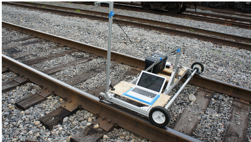
Figure 3-3 Scanning cart with laser processing system on-board
