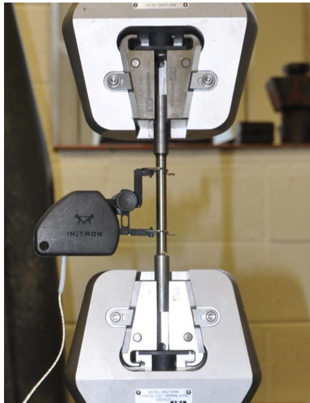
Figure 3-41. Tensile Test Specimen with Extensometer
