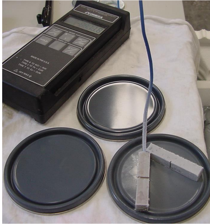
Figure 3-43. CVN Specimen Reaching Desired Test Temperature
