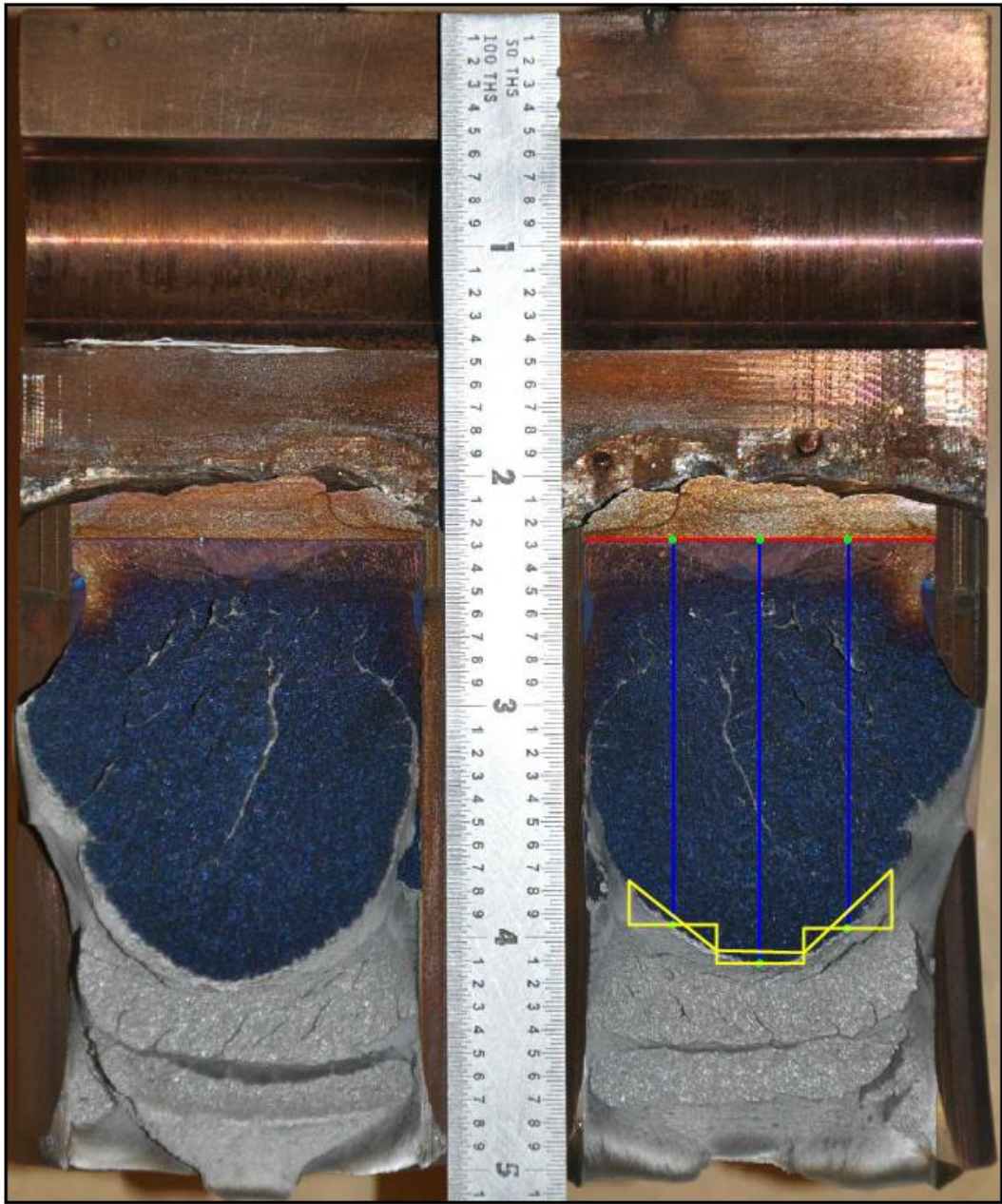
Figure H-14. Specimen D7a Fracture Surface
