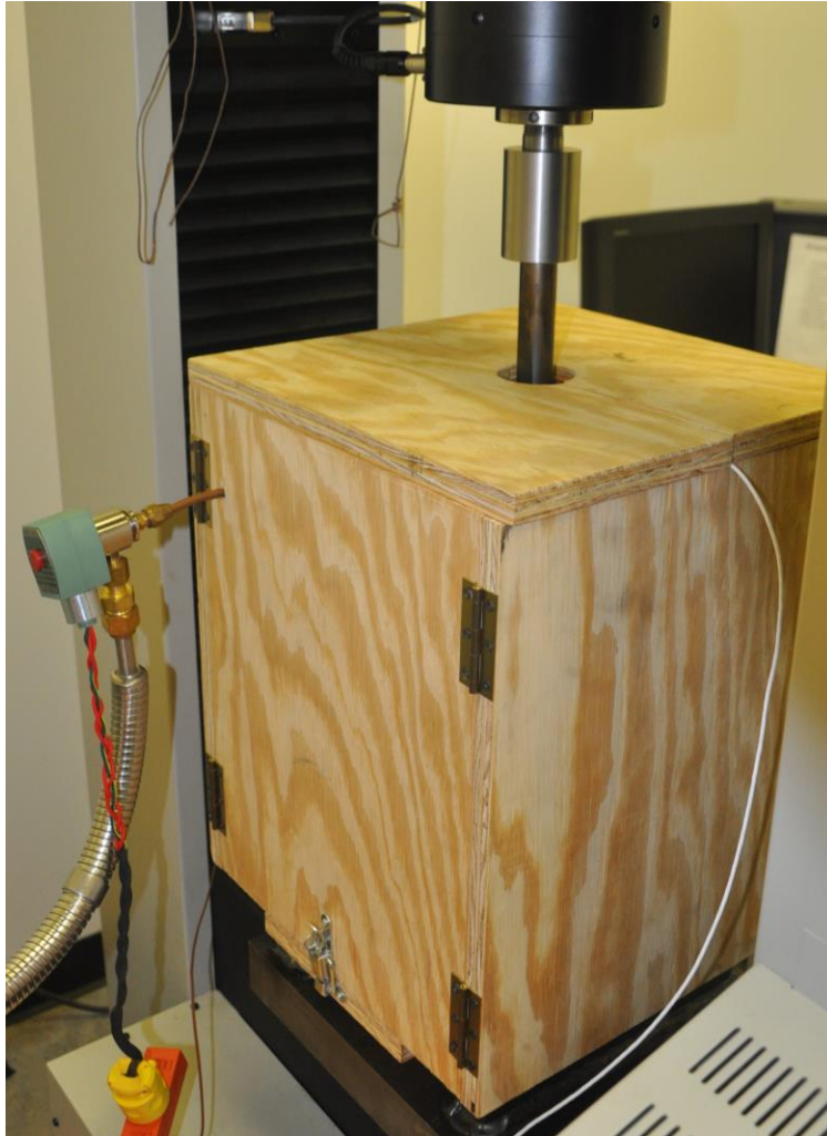
Figure 3-52. Environmental Chamber on Crack Arrest Apparatus
