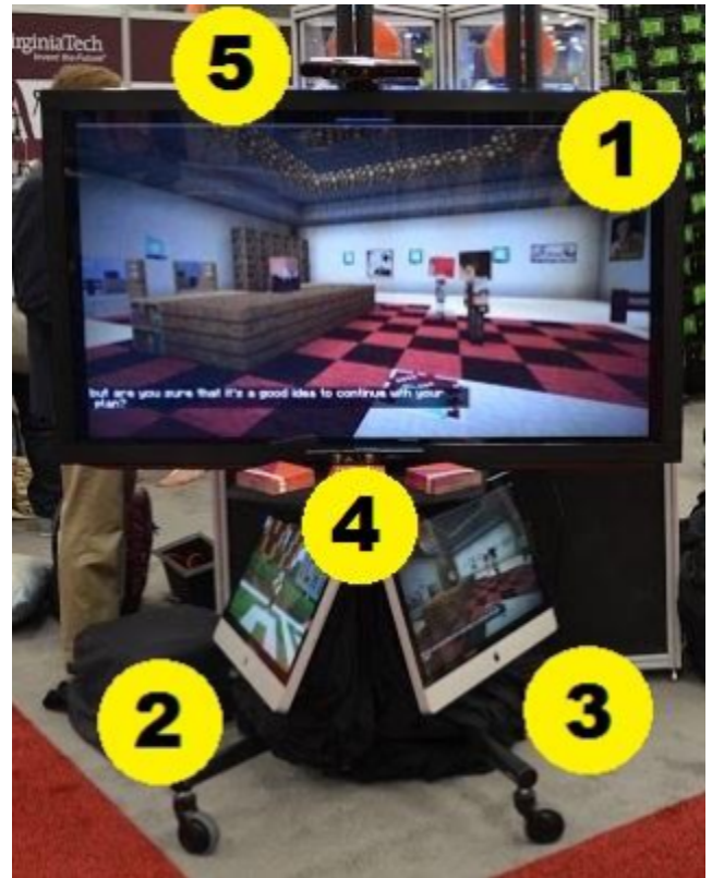
Figure 4.1.2: Prototype Hardware Setup. As labeled, the prototype includes the primary display monitor (1), the computers for collecting data (2, 3), and the Kinect devices (4, 5). This is the SXSW 2016 display.
