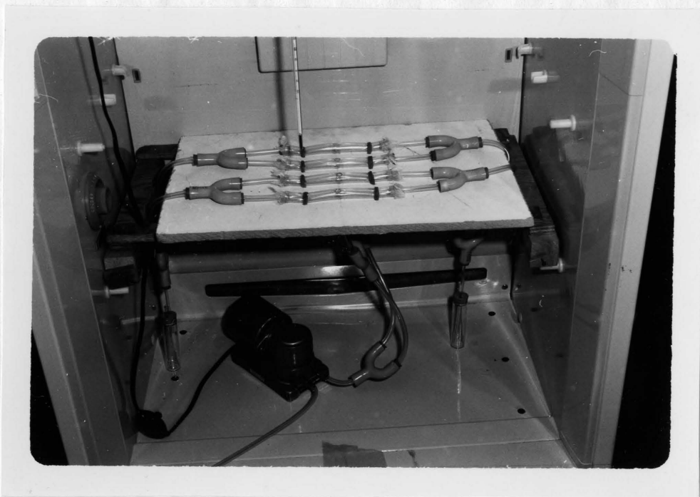
Figure 16. Moving air olfactometer in Basal Oxygen Demand Incubator.
