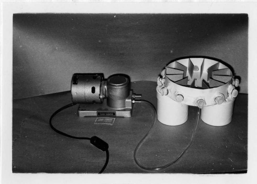
Figure 14. Circular choice olfactometer with air pump.
