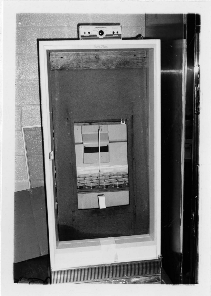
Figure 18. Basal Oxygen Demand Incubator equipped with special masonite and glass observation door.
