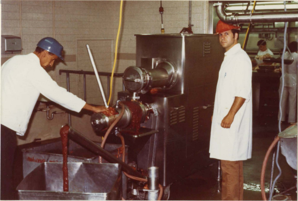
Figure 1. Spleen separation with a Beehive Model AU4171 deboner and desinewing head.
