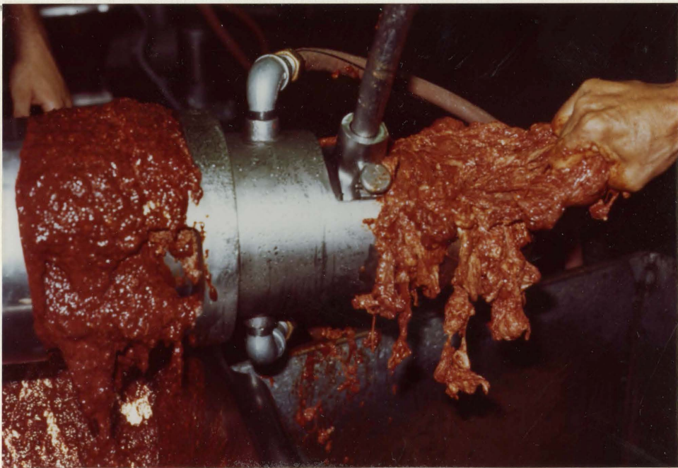
Figure 2. A close-up view of mechanically separated spleen (left) leaving the product port and the residue exiting the discard port.
