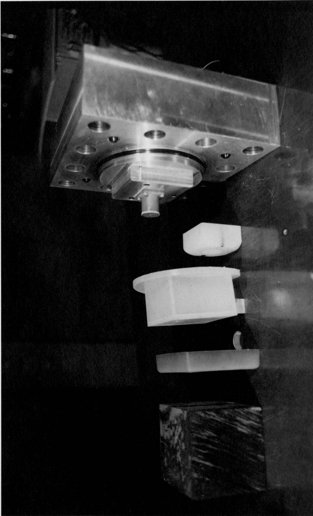
Figure 3.12. Proximity Probe - Exploded View of the Valve
