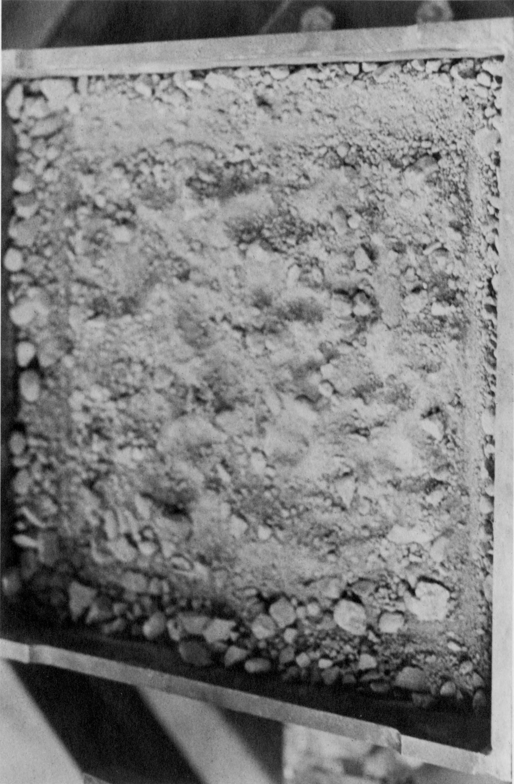
Figure 6.29 Surface of Subballast Bed - After Test
