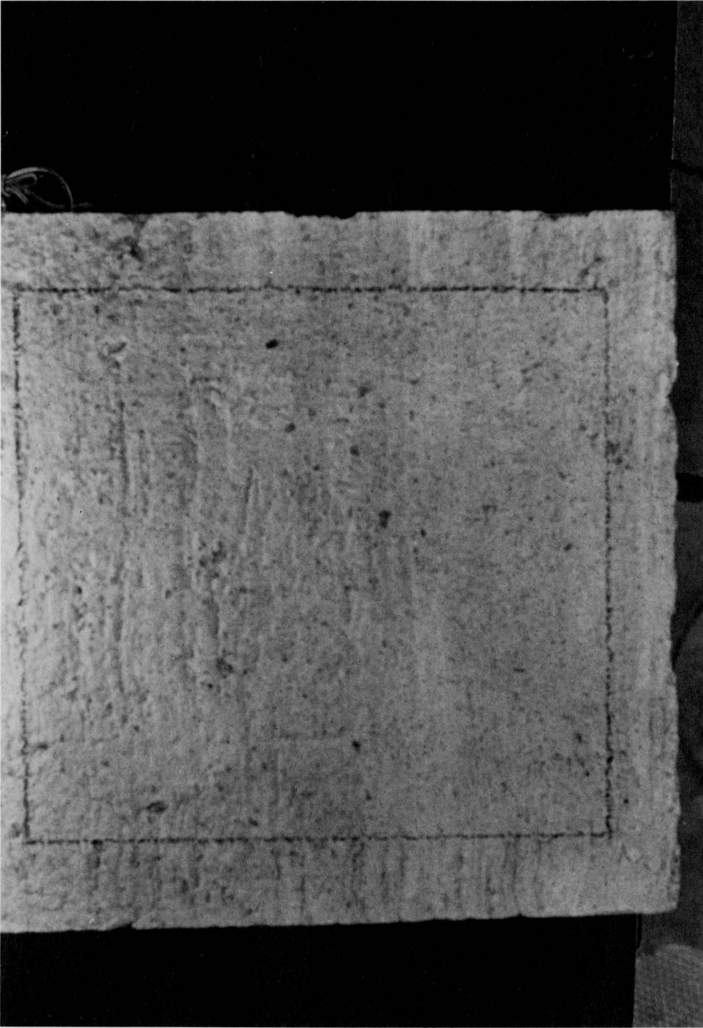
Figure 6.21 Concrete Block Surface - After Test
