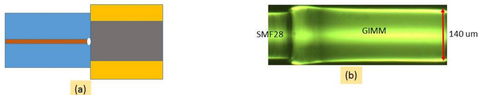
Figure 3.4.3: HF-etched SMF 28 fiber fusion spliced with GIMMF: (a) schematic, (b) micrograph.
