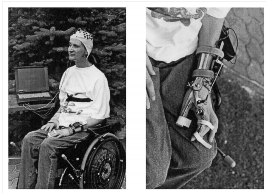
Figure 2.2: Left: tetraplegic patient with portable BCI hardware. Right: Electrically driven hand orthosis on the patient's left hand. [35] [fair use]
