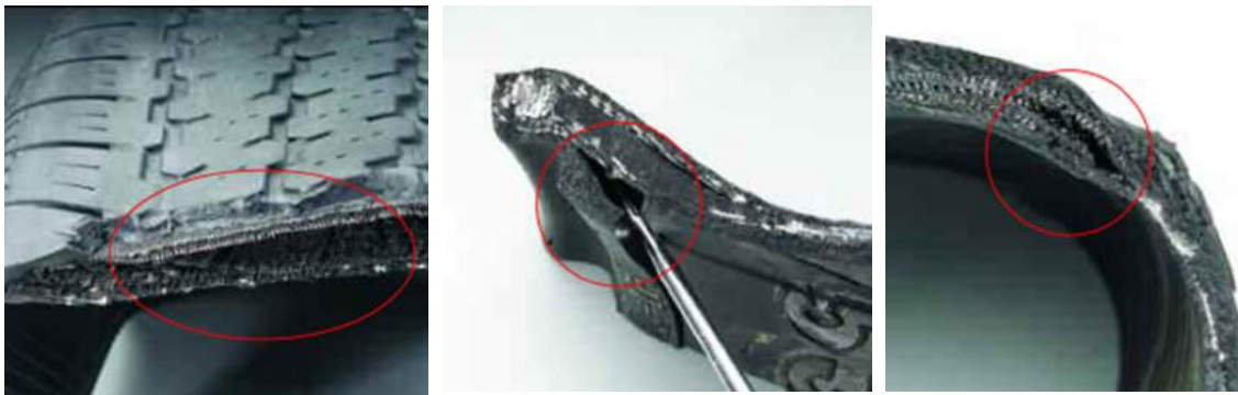
Figure 1.1: Types of non-visually identifiable tire damages; Left: Belt separation; Center: Bead separation; Right: Shoulder Separation [54]
