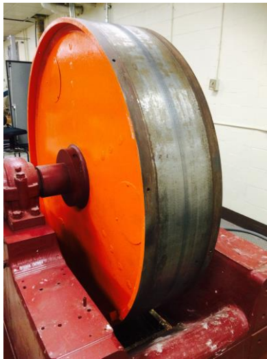
Figure 26: Drum Surface Cleaning using Acetone
