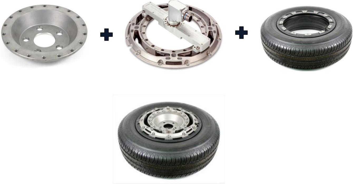
Figure 64: Wheel Force Transducer Assembly – Taken from Michigan Scientific – WFT Presentation
