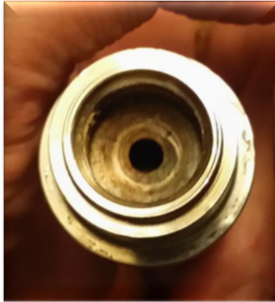
Figure 2. 22 Photograph of an incorrectly sized gas connector having too small
