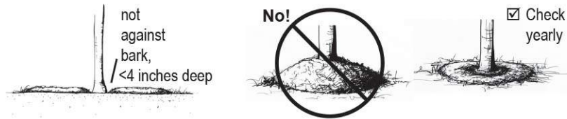
Figure 6: Diagram of proper mulching technique. Image from "Tree Owner's Manual." United States Department of Agriculture, Forest Service, and Northeastern Area State and Private Forestry. www.treeownersmanual.info .
