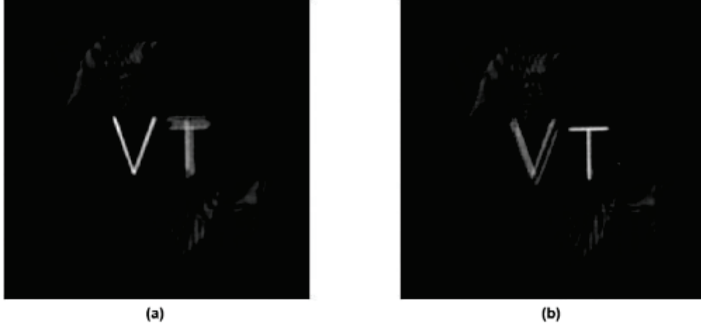
Figure 27 Reconstruction using the pinhole holograms shown Figure 23 and Figure 26 (a) Shows the “V” reconstructed correctly at z_0 = 0\text{cm} and (b) Shows the “T” reconstructed correctly at z_0 = 4.5\text{cm} . [Used with permission]
