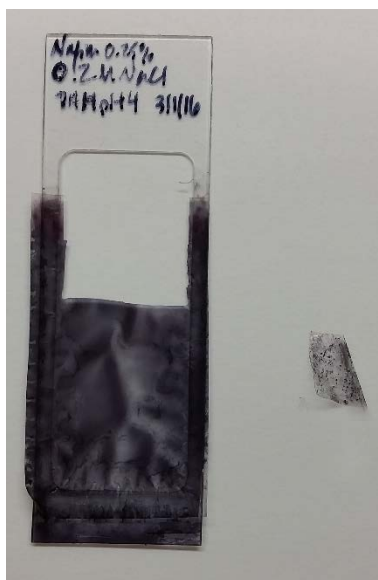
Figure 4.8: Before and after soaking at 80 °C for the 0.2 M NaCl in Nafion sample. The CNC degraded significantly, and wiped off, as shown above.
