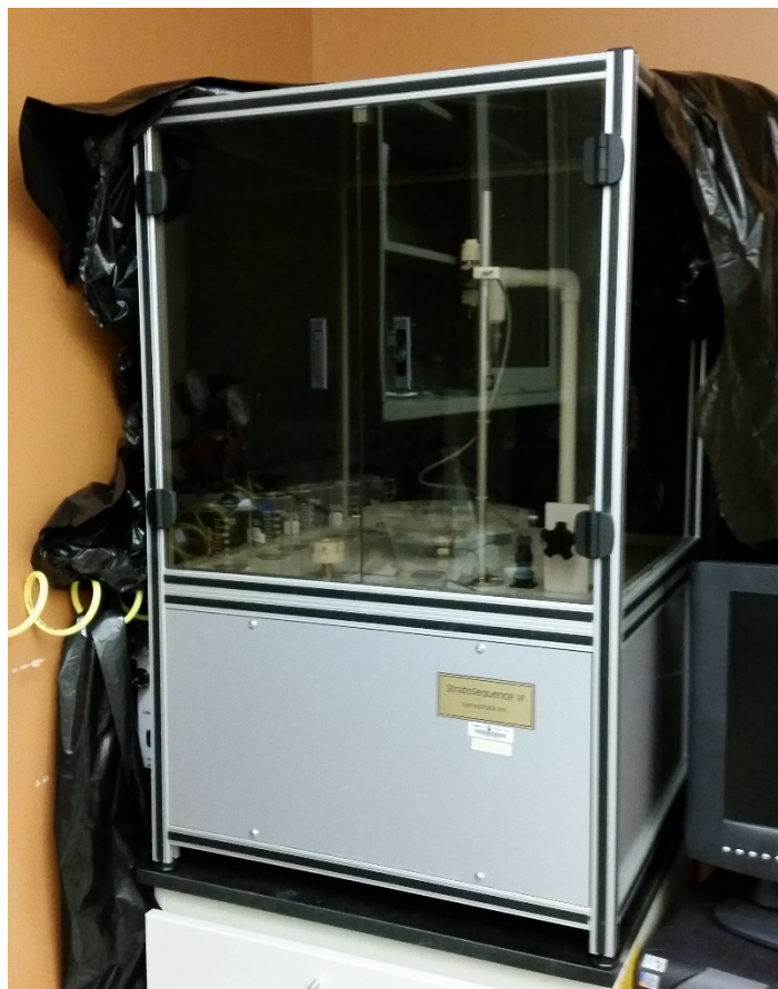
Figure 2.2: Nanostrata programmable dipping robot.
