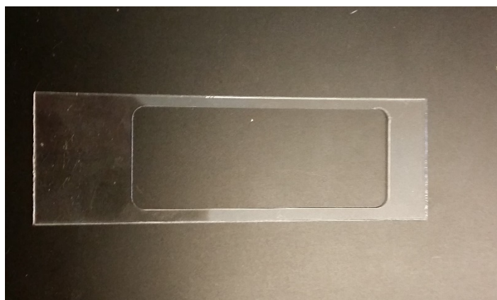
Figure 2.1: Plastic frame used for mounting Nafion films during LbL film deposition.
