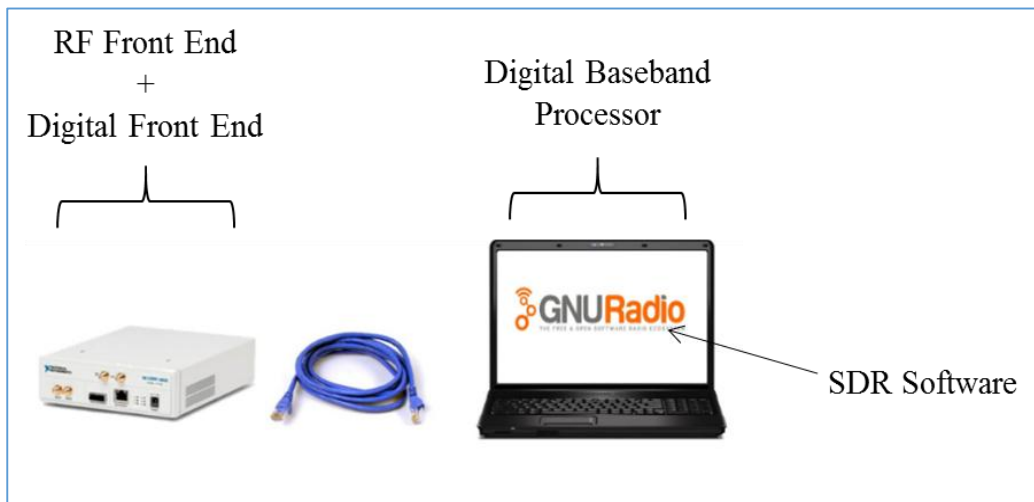
Figure 2.3: SDR System w/ USRP and GNU Radio
