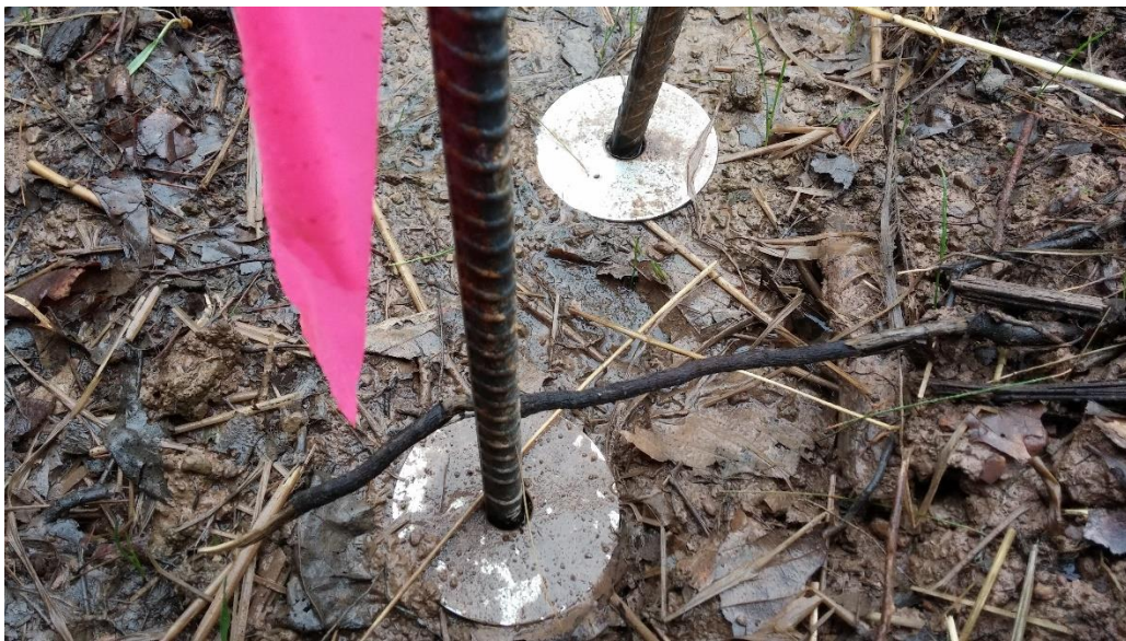
Figure 2.5: Pins in silt fence sediment trap. Washers were placed loosely about the shaft of each pin and made flush with the surface of the ground. Washers allowed data collection to be more easily and accurately conducted by separating the surface of the ground from the collected sediment.
