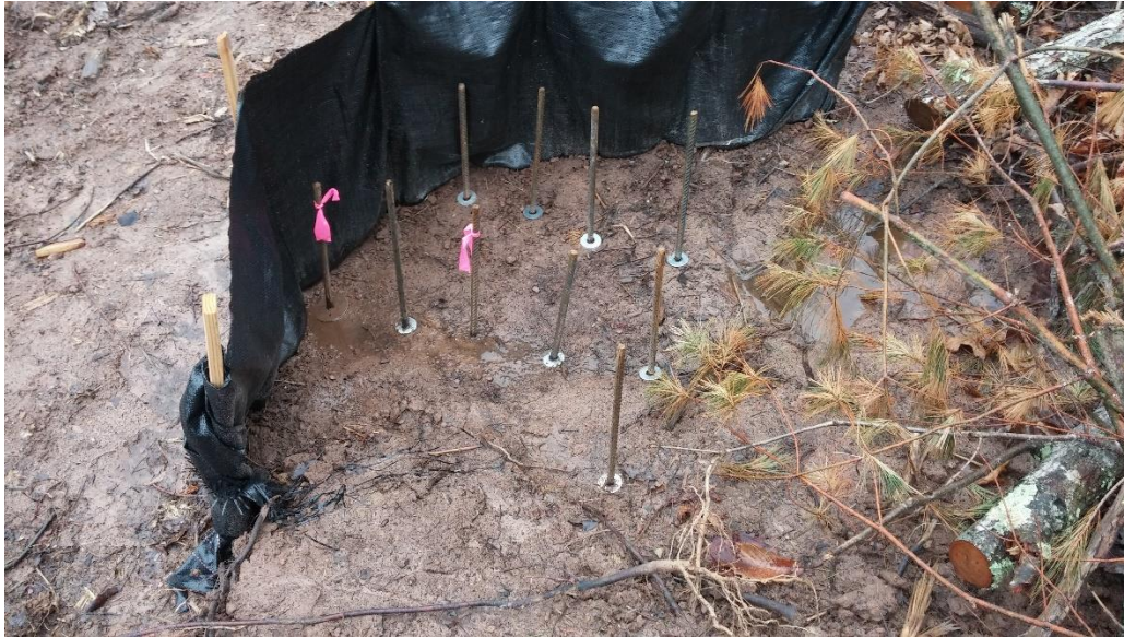
Figure 2.4: Sediment trap with erosion pins in place. Note that the pins were arranged in a grid-like pattern, ensuring that each pin represents a specific amount of area on the ground.
