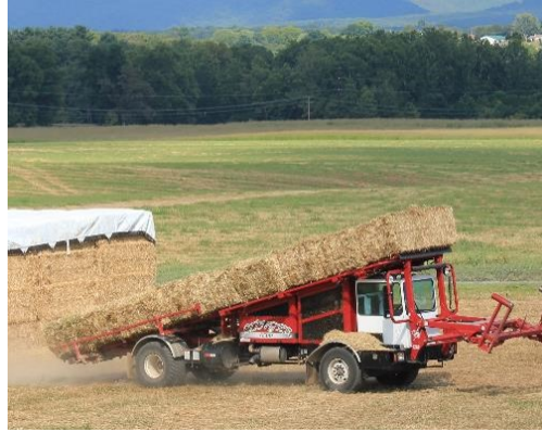
Figure 2.5: In-field hauling of large rectangular bales. ( Source: Antares Group )
