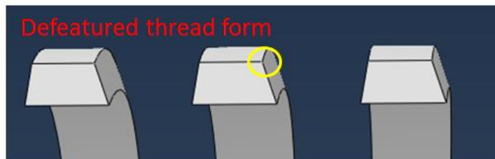
Figure 3.5: Helical threads are defeatured by removing edge radius (top). Cut view of the modeled defeatured helical thread form (bottom).
