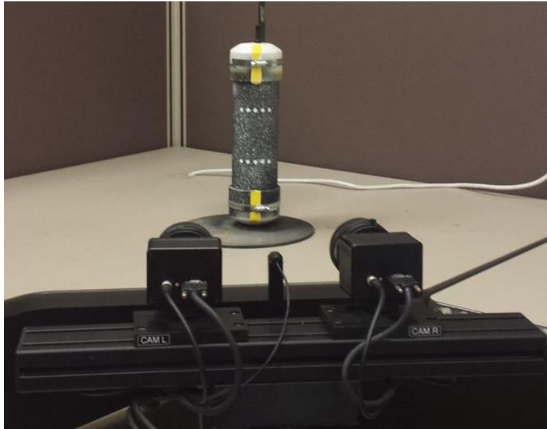
Figure 4.11: Pressure cylinder DIC experiment set up.
