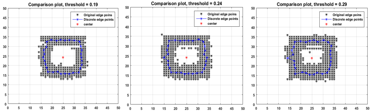
Figure 4-37: Comparison between original edge points and estimated edge points on pothole with gradual edges developed from Expected Distance Edge Detection Method
