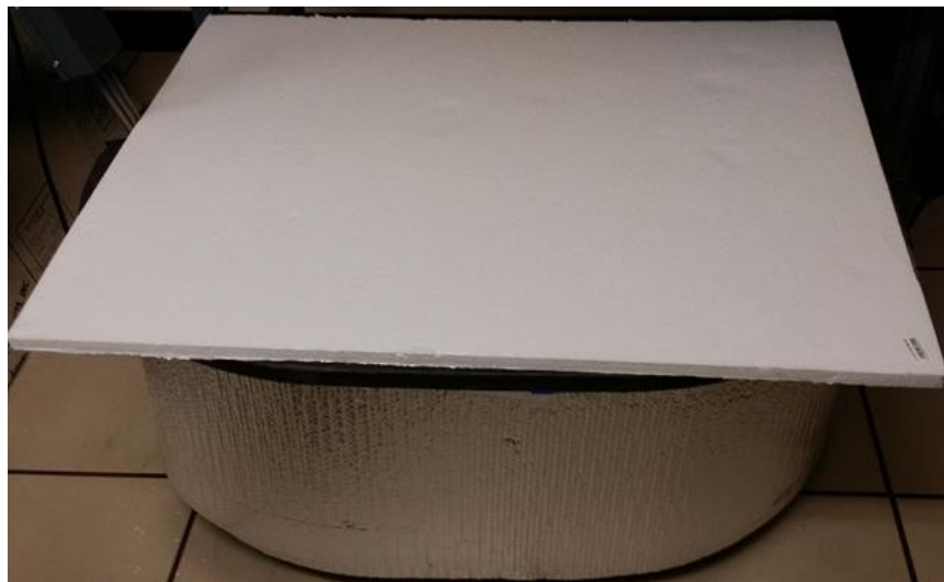
Figure 8: Insulated battery water bath.
