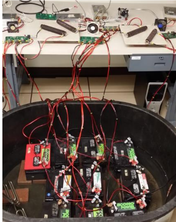
Figure 7: Battery aging test bench.
