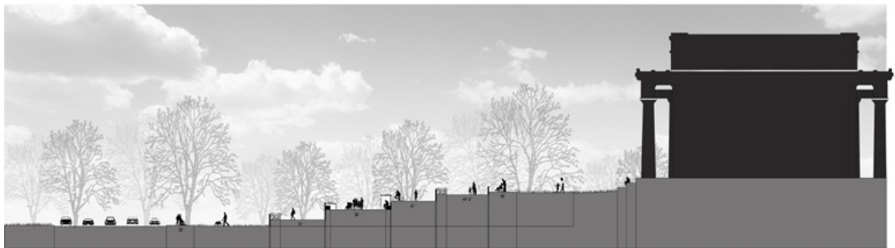
Figure 32 - Section displaying the proposed re-design of the western side of the Lincoln Memorial, providing an alternative and accessible entrance.
